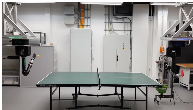
Fig. 1: Robot table tennis setup used to evaluate the proposed methods. We use four cameras attached to the ceiling to track the position of the ball. The robots used are two Barrett WAM robot arms capable of high speed motion, with seven degrees of freedom like a human arm.
