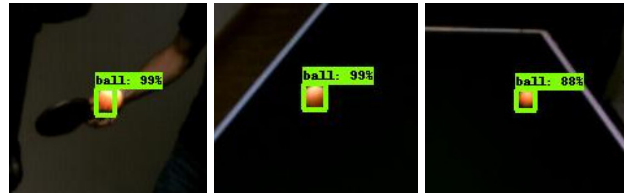
Fig. 2: Ball detection with a Mobilnet deep network architecture using the Single Shot Detection (SSD) method. Note that the SSD method finds the location of the ball in all the images with relatively good accuracy. However, we obtain an average of 15 ball observations per second on a four camera setup, not efficient enough for a highly dynamic task like robot table tennis.
