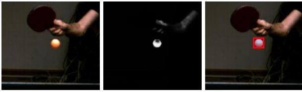
Fig. 3: Ball detection using a single convolutional unit in a semantic segmentation setting. The image on the left shows a section of a table tennis scene. The image on the center shows the probability image \mathbf{B} representing the probability assigned to each pixel of being the ball. Dark means low probability and bright means high probability. The image on the right shows the detected ball position. This simple model can successfully find the ball in the image, and it is around 50 times faster than the SSD method.
