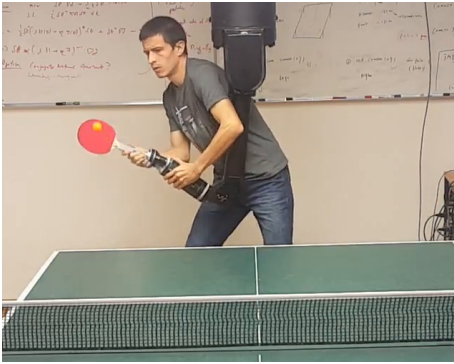
Fig. 10: A human subject moving the robot in gravity compensation mode. Gravity compensation mode was used to obtain the human demonstrations necessary to train the robot.
